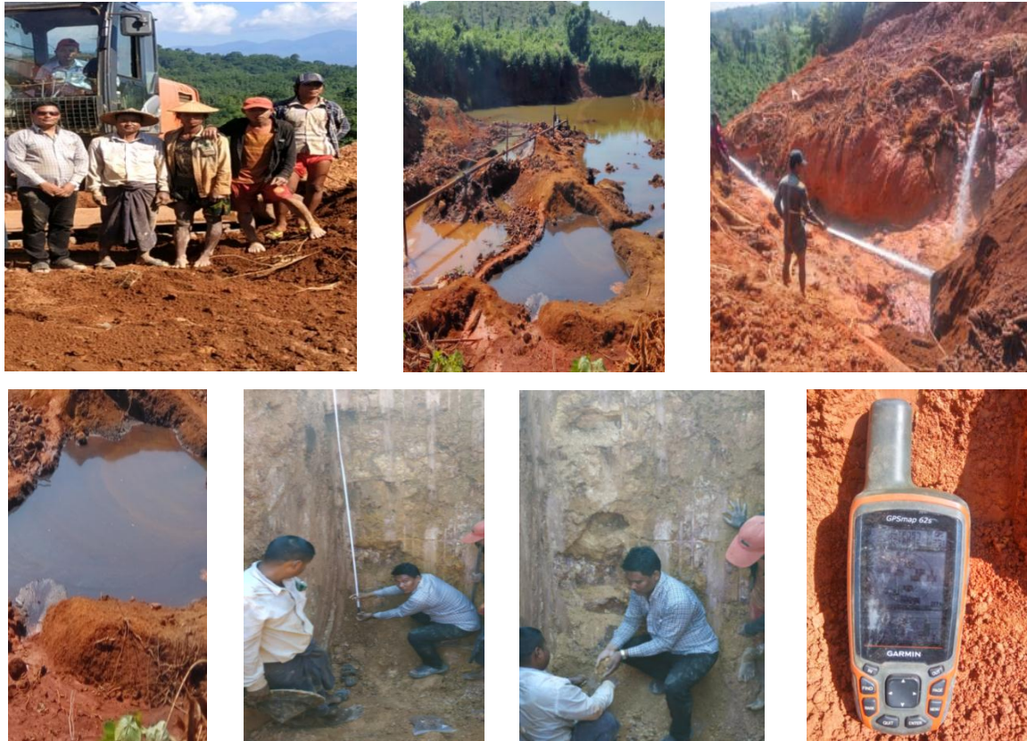
Figure 4 Photo graph of taking the sample of the soil and water on various depths
